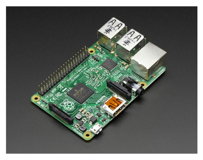
Best of all, the Pi 2 keeps the same shape, connectors and mounting holes as the Raspberry Pi B+. That means that all of your HATs and other plug-in daughterboards will work just fine. 99% of cases and accessories will be fully compatible with both versions
